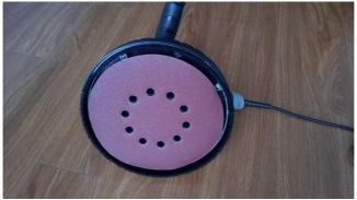
Remove the sandpaper, put the Allen wrench into the hexagon hole in the center of the viscid disc and then rotate clockwise to take off the damaged viscid disc. Install the new viscid disc (see the picture).
