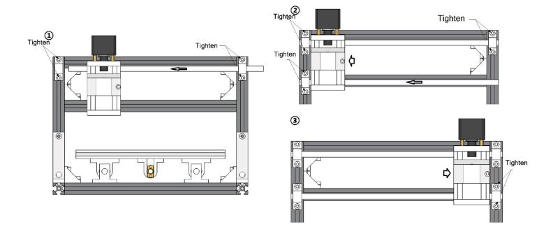
i. Lead screw installation: 400mm X-axis Lead screw x1, 320mm Y-axis Lead screw x1, Copper nut x2, Spring x2
