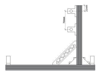
f. Y-axis installation: Bolt M5\*10×10, Slide nut 30M5×10, Y-axis slider x4, Y-axis nut seat x1, 330mm Linear axis x2, Mesa×1 (Elevation view)
