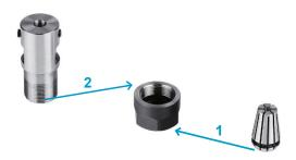
2. Install the ER11 extension rod holder into the motor. Generally, it's a little difficult to install. Installation: The aperture is smaller than the actual 0.02mm. According to the high-frequency heating (300 degrees Celsius), thermal expansion and contraction principle, to expand the hole, then insert the spindle and lock it, and then fix the shaft collet after cooling completely.
