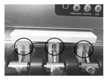
(4) Install the handles to the valve stems one by one ,in the mean time, slowly push the steel pin through the discharger and the handles. (Refer to below photo for the correct direction of the handles)
